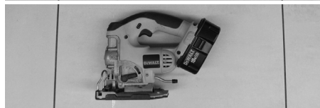
16 A Jigsaw OR a Sawsall can be used to cut the opening.
